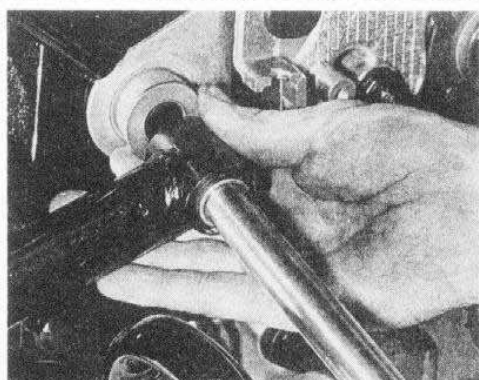
12.2 Do not omit thrust washers when refitting swinging arm
