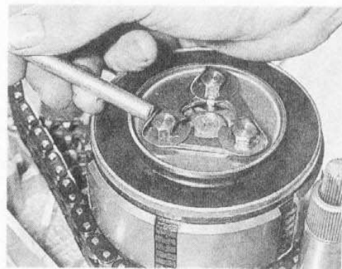
33.7c ... and bend up the tab washers
