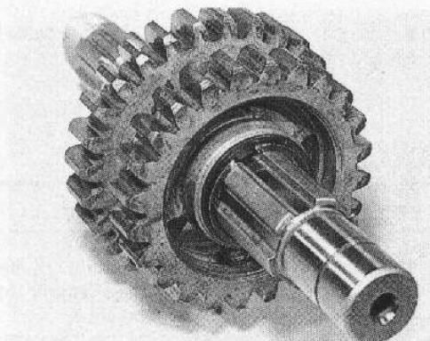
26.13c ... and secure all the above components in position with a circlip
