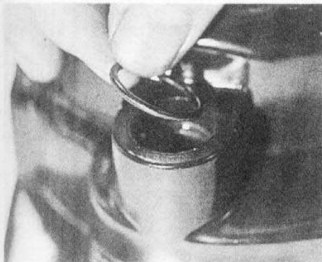
34.1a Check condition of cover O-ring, renewing if necessary
