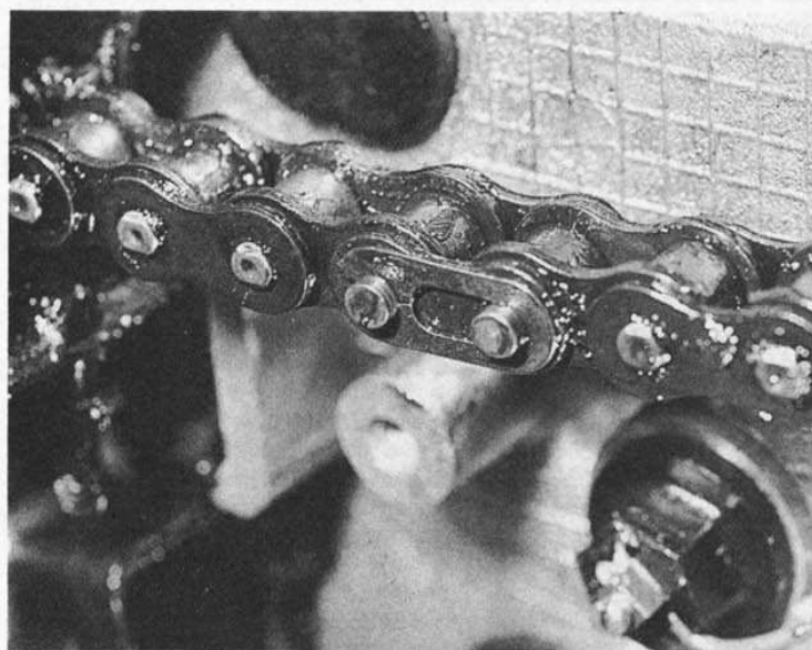
Refit spring clip with closed end in normal direction of travel
