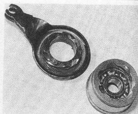
22.7 Examine clutch lifting mechanism worm gear for wear - 251 shown
