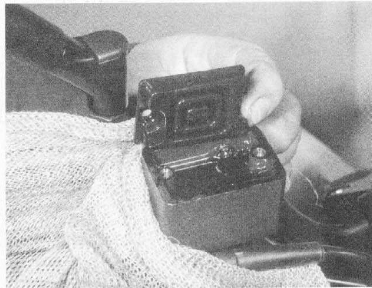
2.2b Remove reservoir cap, plate and diaphragm to add fluid
