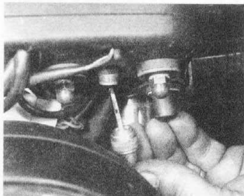
10.3 Unscrew its knurled ring and detach speedometer cable
