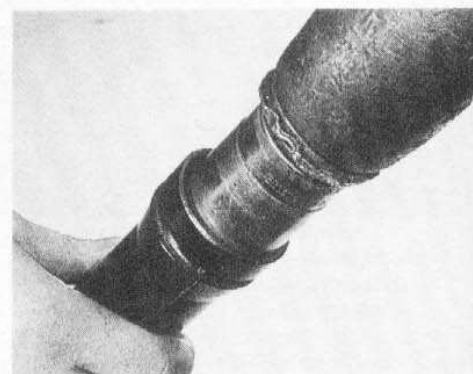
3.8a Tap fork seal into position using a suitable size tubular drift
