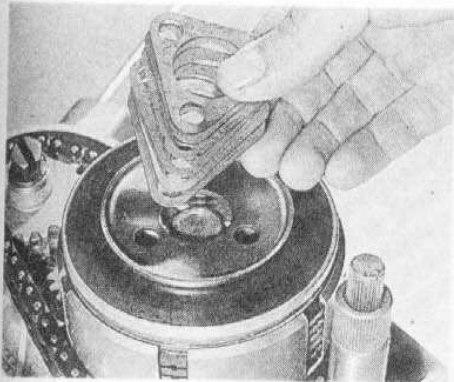
33.7a Calculate and fit the required amount of shims ...
