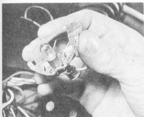
13.2b ...remove bulb retaining plate and parking lamp bulb...
